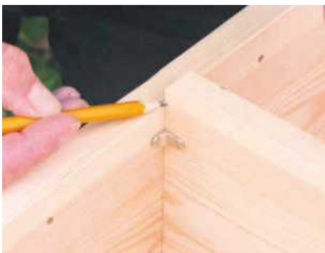
STEP 19. Mark the shelf depth and saw both pieces to width. You may need to trim the ends if too tight
